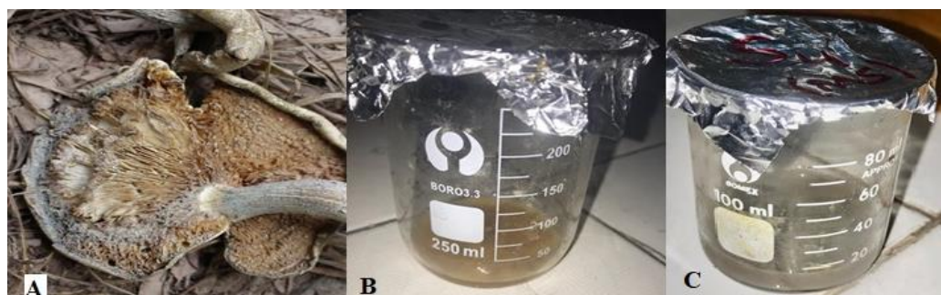
Fig.4. (A) Lepista sordida ; (B) Lepista sordida extract and \text{AgNO}_3 ; (C) synthesized silver nanoparticles (AgNPs).
