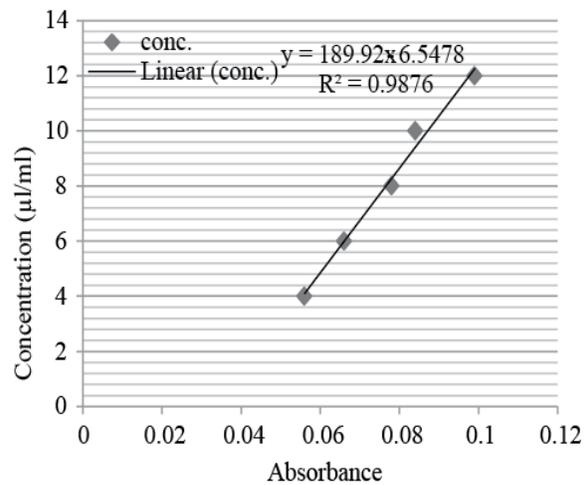
Fig. 6. Absorbance of standards for guaiacol used in peroxidase assay observed at 470 nm wavelength.
