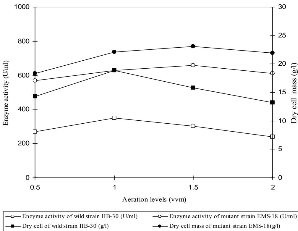
Fig. 3. Effect of different aeration levels on the alpha amylase production by *A. oryzae* IIB-30 and its mutant derivative *A. oryzae* EMS-18 \*
