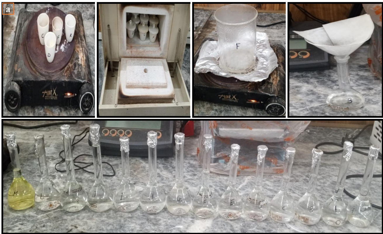
Fig 2. Acid digestion of flour blends for mineralization analysis through Atomic Absorption Spectroscopy and Flame Photometer a. Charring, b. Ashing, c. Acid digestion, d. Filtration, e. Flour blend samples
