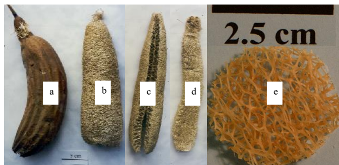
Fig. 1. (a) Matured dried fruit of Luffa cylindrica , (b) Loofa sponge recovered from (a) after removing the hard cover of the fruit, (c-d) longitudinally cut pieces of loofa sponge, (e) sponge discs (2.5 cm in diameter) showing multilayered fibrous network.
