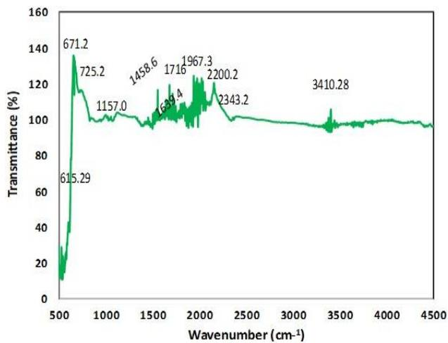
Fig. 2. FTIR analysis of ZnONPs.
