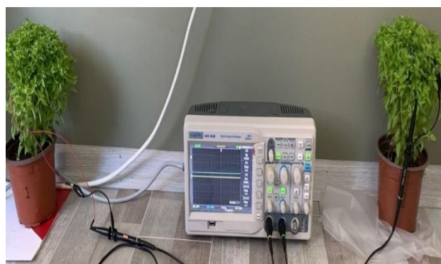
Fig. 3. Frequency and electrical voltage measurement of O. basilicum L. in indoor (Social distance position).
