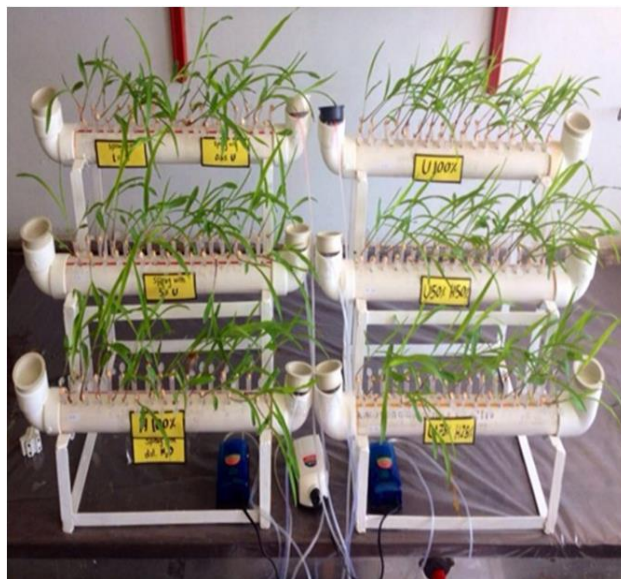
Fig. 1. Polyethylene tubes used in the study as hydroponic growth units.
