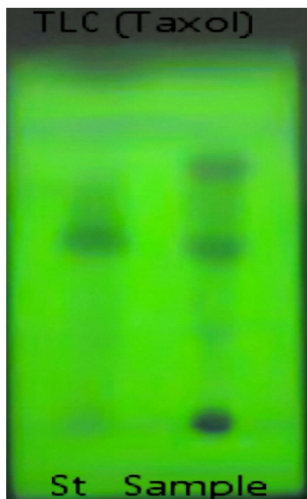
Fig 1: TLC plates showing taxol in fungal culture broth
