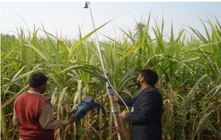
Fig. 2. Cropscan Multispectral Radiometer (MSR5) at study area.
