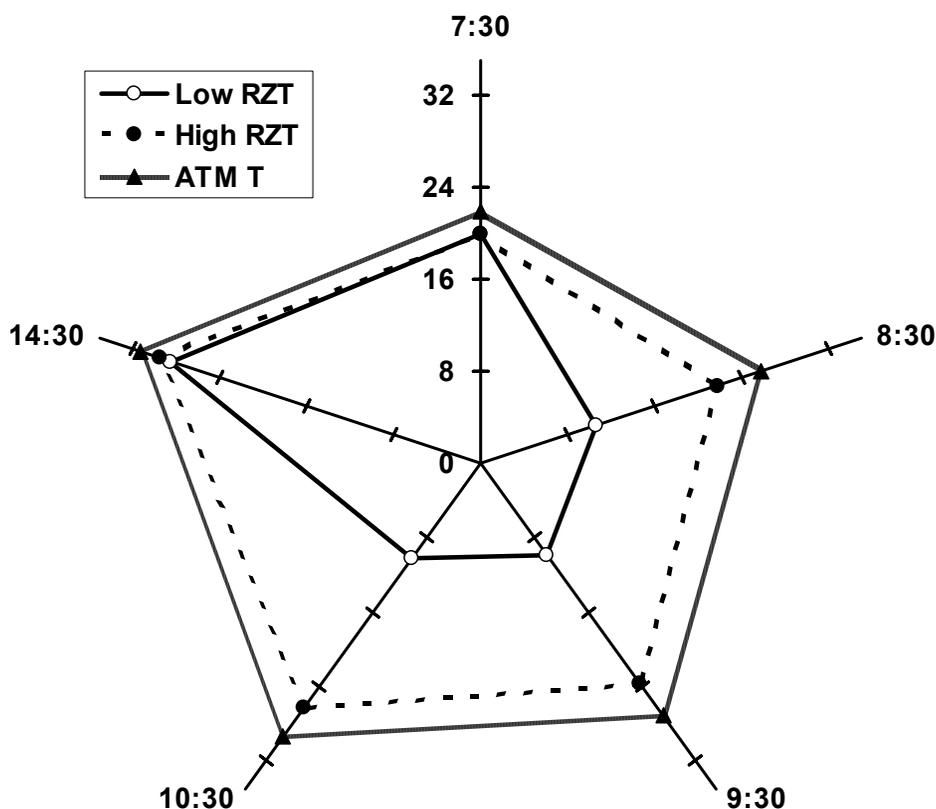
Fig. 1. Daily cycle of low root-zone temperature (RZT), high RZT (ambient) and atmospheric temperature (ATM T) of pots and greenhouse measured in Celsius scale ( $^\circ\text{C}$ )
