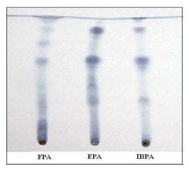
Fig 4. Typical TLC chromatogram of phenolic acids in seeds of Barri 2000. FPA: Free phenolic acids, EPA: Esterified phenolic acids, IBPA: Insoluble-bound phenolic acids. Adsorbent material: Silica gel, Solvent system: chloroform-acetic acid (9:1; v/v), Locating reagent: Folin-Ciocalteu reagent.
