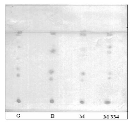
Fig. 2. TLC chromatograms of tannins in different groundnut varieties. G; Golden, B; Barri 2000, M; Mongphalla, M 334; Mongphalli 334, Adsorbent material: Silica gel, Solvent system; chloroform-acetic acid (9:1 v/v), Locating reagent; Folin-Ciocalteu reagent.
