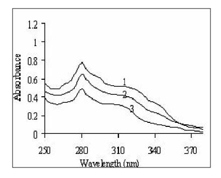
Fig. 3. Typical UV spectra of methanolic solutions of different phenolic acid fractions in the seeds of Barri 2000. (1) Insoluble-bound phenolic acids, (2) Free phenolic acids and (3) Esterified phenolic acids, Wavelength range 250-380 nm.
